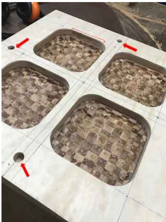
Board with template after forstner bit use. Arrows indicate indexing holes
