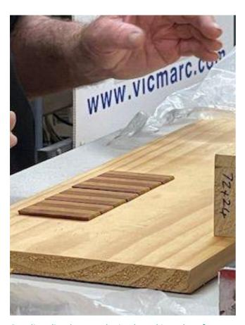
Cut slices lined up on glueing board in order of cut
