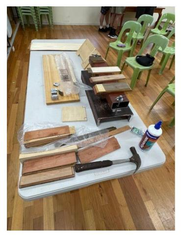
Laminated blocks prepared for slices using jig and bandsaw/dropsaw
