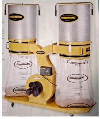
Powermatic PM1900 Dual Dust Collector with pleated cartridge filters. This is a 2014 model but in as new condition.
