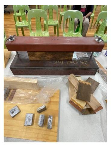
Table set out with the pre-made laminated blocks, cramp, gluing board, plastic and metal weight.
