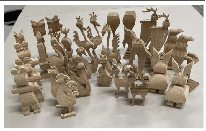
For some years now, at irregular times, I have cut compound patterns on the scroll saw. These were mainly in the form of a pattern as seen in the photo at right. However each image is limited to the depth of cut of one's scroll saw. In my case that's about 45mm.
