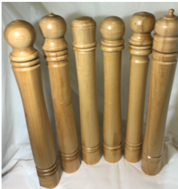
Lionel Hart is making a variety of Pepper Grinders using 100 year old Spruce from ex piano frames. The finish is Nitrocellulose.
