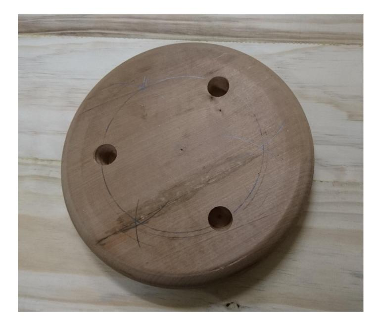
George says: ' there is no exact angle for the leg-seat socket, it depends on the leg length which is set by the seat height that you want. The seat diameter should be slightly less than the circle made by the leg tips. The stool should also look balanced and be stable in use. A few variables to play with as you make a prototype or use scrap wood to test some options'.
