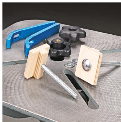
These simple hold-downs are custom fit to the slots of your drill press table. Two of these clamps will cover all your needs.
