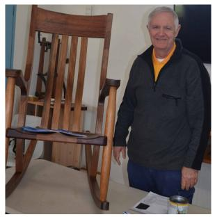
ple, and Rosewood. The rockers, back legs, splats and crest rail are all cold glue laminated using MDF bending forms.
