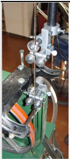
14" Hafco Our old Bandsaw has had a bit of a facelift during this last month. The upper and lower blade guide bearing have been replaced as seen in the photo by a set of Baladonia Tools Bandsaw Blade Deluxe Guide Set.
