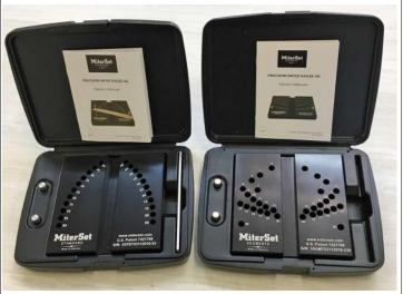
Do you want to cut accurate mitre cuts on our table saws, band saws and router tables then our Club's latest acquisition is ready for you to try out. It not only allows you to cut 45 degree mitres but enables you to accurately cut the correct angles for multi sided items from four to 12 sided.
