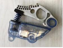
The photo at left is of a triggered cartridge from one of our Sawstop Table Saws. We have had to replace two of these in the last month. No, on either occasion did the triggered cartridge saved a finger or a hand.
