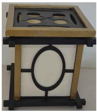
In this case the frame is recycled Radiata pine; while the panels are plywood. The frame joints are all half lap that I cut on the table saw.
